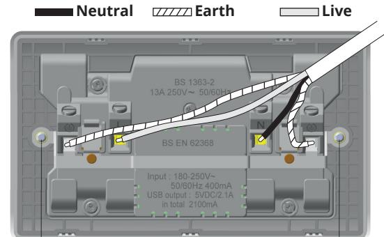
Although the product has twin earth terminal it will function with one earth connected.
